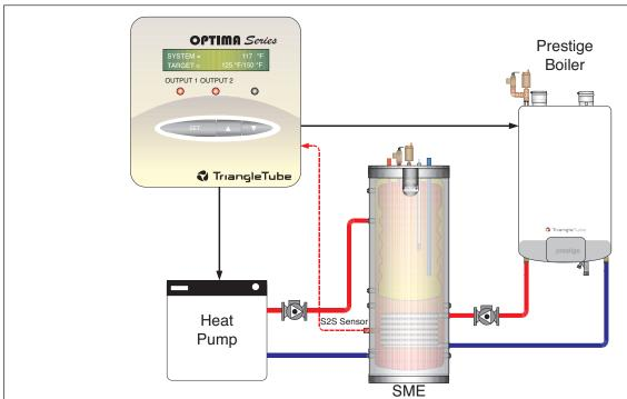
S2S Application: The S2S monitors the SME temperature and stages on the Heat Pump and Prestige
