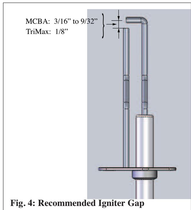
3. Remove any white oxides accumulated on the electrode using fine grit sandpaper or steel wool. If the electrode does not clean to a satisfactory condition, replace the igniter.
