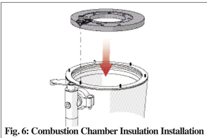
16. Check combustion chamber insulation alignment with the burner mounting plate. The combustion chamber insulation igniter cutout should align with the opening in the burner mounting plate. If not properly aligned, remove the burner mounting plate and reposition combustion chamber insulation.
