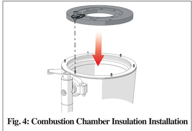
**Fig. 4: Combustion Chamber Insulation Installation**
