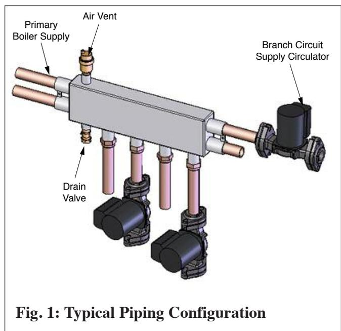
**Fig. 1: Typical Piping Configuration**
